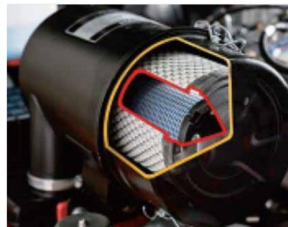
Optimized air intake and exhaust system, high-capacity exhaust silencer and high-effect intake muffler will reduce the noise of full truck by 3dB and reduce the vibration by 20%.
