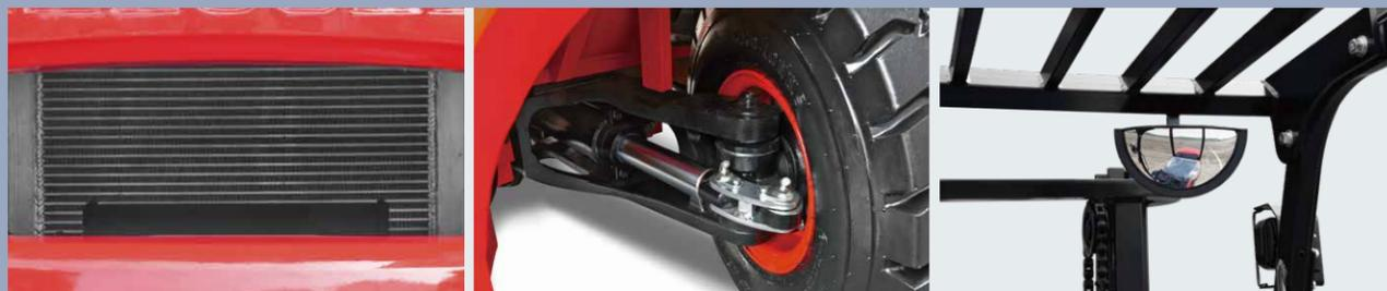
1. The radiator adopts aluminous plate-fin radiator with better performance and higher structural strength independent oil radiator, optimized oil and water heat dissipation channel and double ventilation holes on counterweight can greatly improve cooling efficiency and reliability of overloaded operation and ensure reliable operation of the engine.
